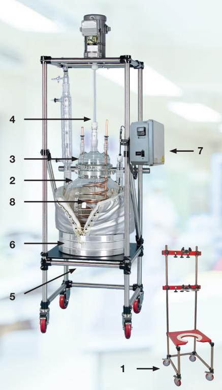
Universal open frame stand design allows for maximum clearance and access to the ports on the head. To allow for scale up, the frame has been designed to be fitted with vessels from 10L to 200L in size. For versatility, our systems have been designed with a working temperature range of ambient through 200°C, and wetted surfaces of borosilicate glass and PTFE.
