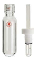
Heavy wall tube with bushing and plunger valve that allows purging of the tube. Closed bottom plunger has a hole inside, that when positioned in relation to O-Ring seal, will open Tube to the atmosphere (i.e.,
