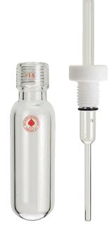
Rugged, heavy wall tube, similar to listing above, except glass plunger valve has a 5mm I.D. thermowell for a thermocouple wire or sheathed probe up to 1/8" (3.2mm) O.D. Closed bottom plunger has a hole inside that when positioned in relation to O-Ring seal, allows Tube to be open or closed to the atmosphere (i.e., pull to close, push to
