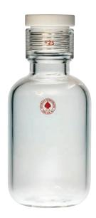
These heavy wall bottles are unique in that Ace-Threds allow for easy closing of plugs, which are reusable. The plugs have O-rings for assurance of a tight seal by simply hand tightening. The bottles are offered in several lengths with #7, #15, #25, or #36 Ace-Threds. They can be custom fabricated in various lengths and diameters, if needed.
