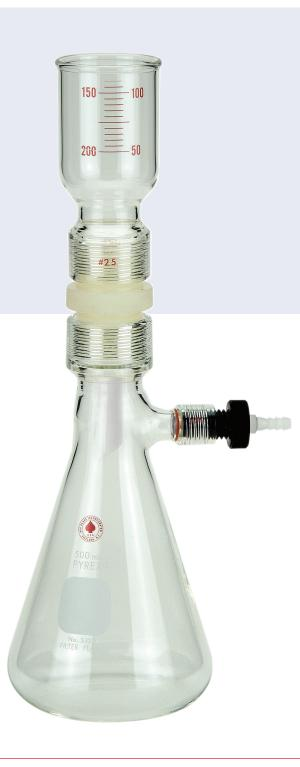
A safer, more stable solution to Vacuum Filtration from Ace Glass. Out with silicone stoppers, collars and clamps. In with Ace-Thred™ funnel to filter flask couplings and Ace-Safe™ hose connections. Not only does the threaded connection between the funnel and the filter flask increase the effectiveness of the vacuum seal, it also offers a rigidity between the two that will increase the safety aspect of the entire apparatus if chain clamped to a stand.
