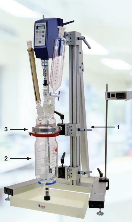
Ace Glass Scale-Up Series<sup>™</sup> reactor systems enable the researcher to scale-up from 100mL to 6000mL on the bench and enjoy the same geometry when replicating those results in our Kilo Scale reactors. Simply select the capacity you desire in the base system seen below. Complete your system with any of the many optional components we offer.
