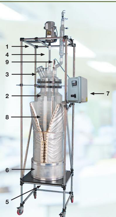
Black epoxy-coated aluminum flask support plate is adjustable vertically, to allow room under flask for various outlet receptacles. Plate is supplied with three adjustable braces to hold mantle in place. Upper support brackets supplied to stabilize flask.
